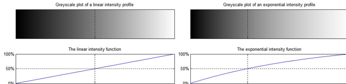
**Figure 1** Linear intensity profile image and corresponding value plot with 50% intensity highlighted (left) versus exponential  $(1 - e^{-(1-x)/\beta})$  intensity profile that better aligns the apparent middle grey level in the centre of the scale (right).
