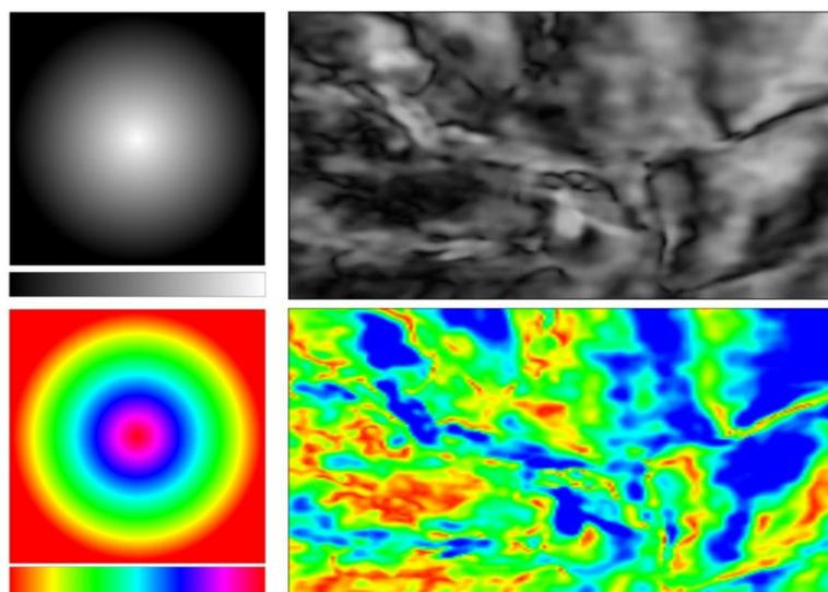
**Figure 2** Left: radial grey-scale pattern uniformly decreasing in amplitude away from the centre (top) and the same image data displayed with a varying hue colour bar (bottom). Right: envelope volume time slice displayed in greyscale (top) and with a spectrum colour bar (bottom).
