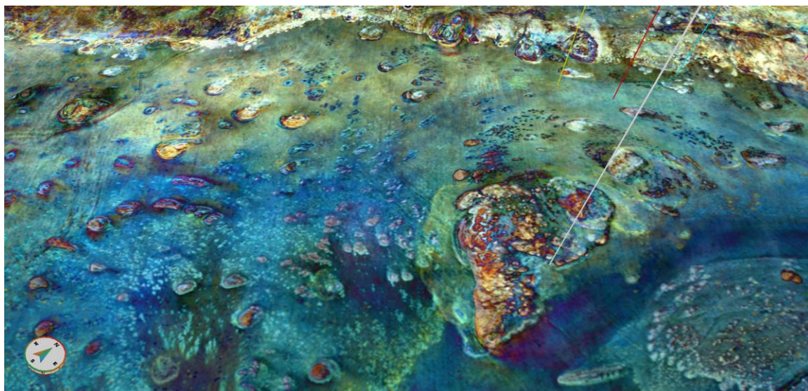
Image. Frequency Decomposition RGB Colour Blend mapped over a horizon surface highlighting carbonate pinnacle reefs and karstification from the Poseidon 3D Dataset in the Browse Basin, offshore Western Australia.
