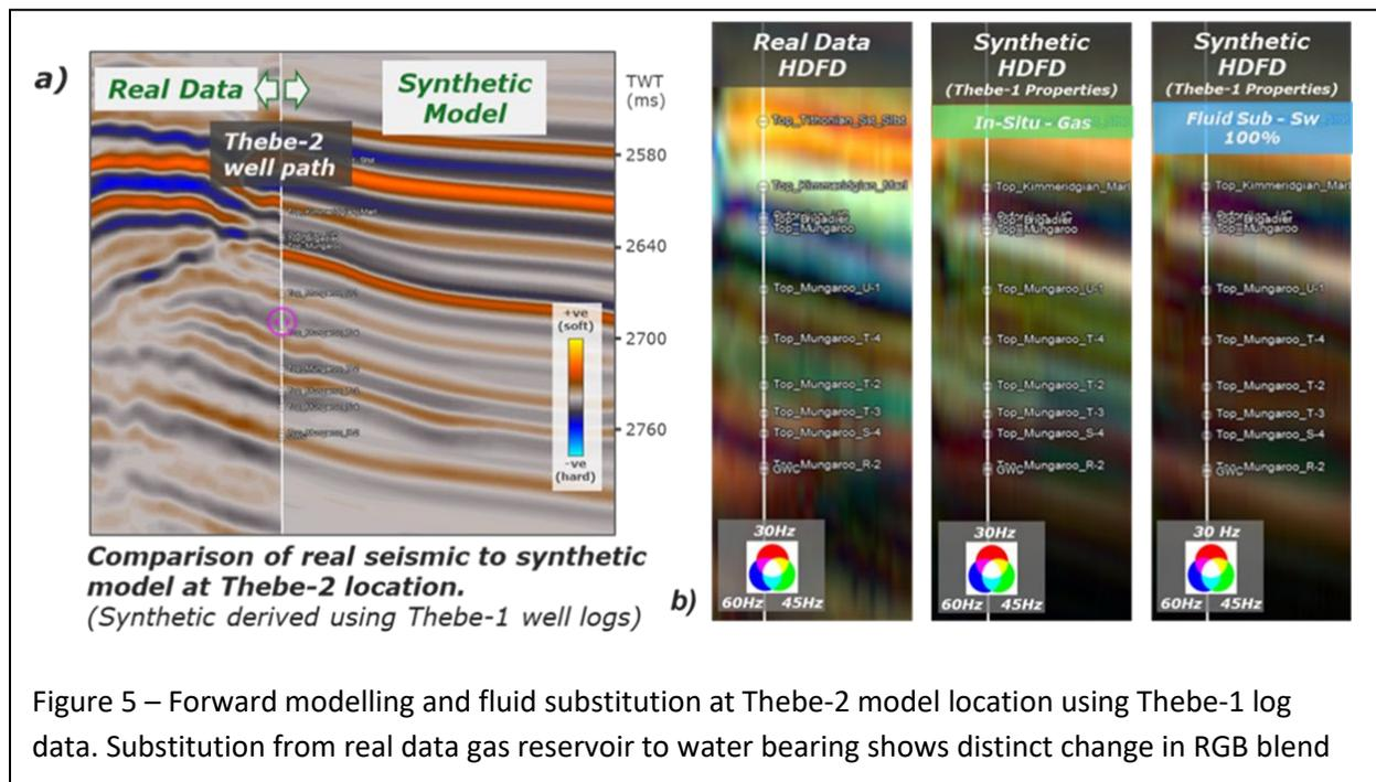
Figure 5 – Forward modelling and fluid substitution at Thebe-2 model location using Thebe-1 log data. Substitution from real data gas reservoir to water bearing shows distinct change in RGB blend
