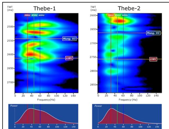
Figure 2: Trace spectrogram showing time-frequency distribution at well locations. Frequency band selection can be tailored around the central frequency at the reservoir interval. In the example the central reservoir frequency of around 45Hz is set as the central (green) band
