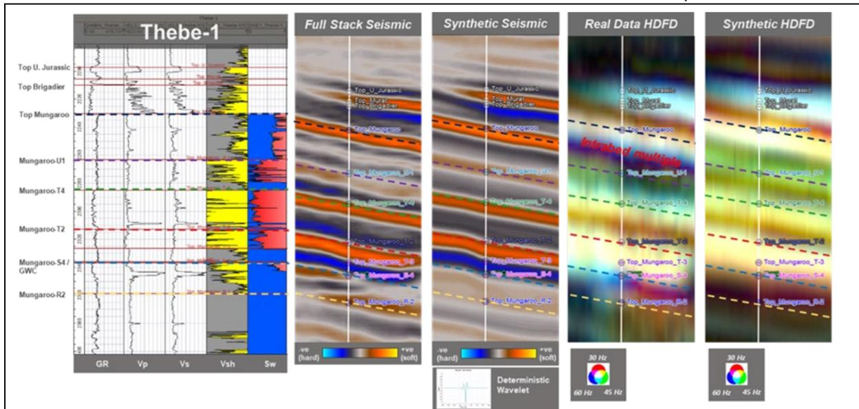
Figure 3: Well correlation at Thebe-1 location. From left to right: well log data, full stack seismic data, synthetic seismic model, High Definition Frequency Decomposition Blend, Synthetic High Definition Frequency Decomposition Blend.
