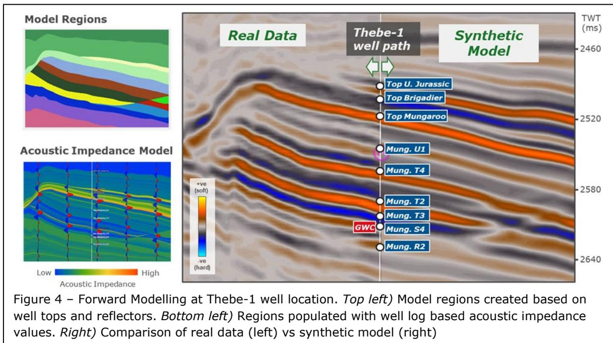
Figure 4 – Forward Modelling at Thebe-1 well location. *Top left*) Model regions created based on well tops and reflectors. *Bottom left*) Regions populated with well log based acoustic impedance values. *Right*) Comparison of real data (left) vs synthetic model (right)
