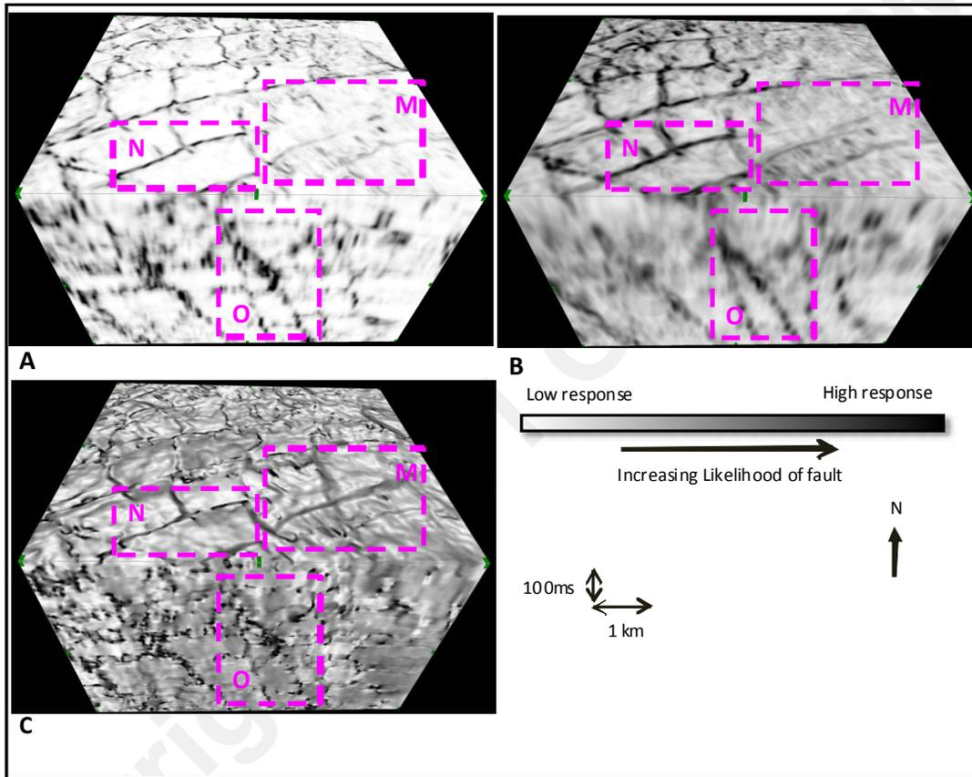
Figure 7. Three fault attributes: (A) structurally oriented semblance, (B) tensor, and (C) dip magnitude.
