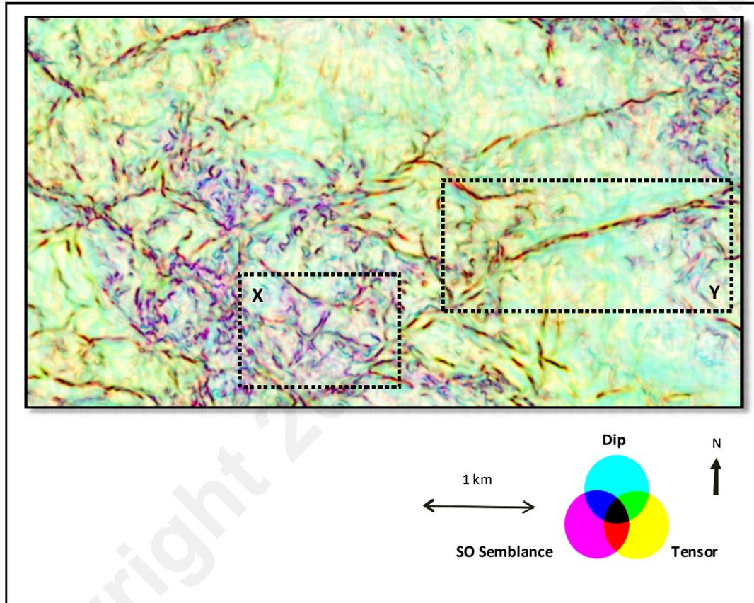
**Figure 5.** The three fault attributes shown in this figure plotted in CMY space forming a blended, multiattribute image of dip magnitude plotted against the cyan axis, structurally oriented semblance plotted against the magenta axis, and tensor plotted against the yellow axis.
