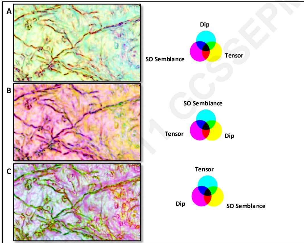
Figure 9. Volume CMY blend of structurally oriented semblance, tensor, and dip attributes associated with different color channels.
