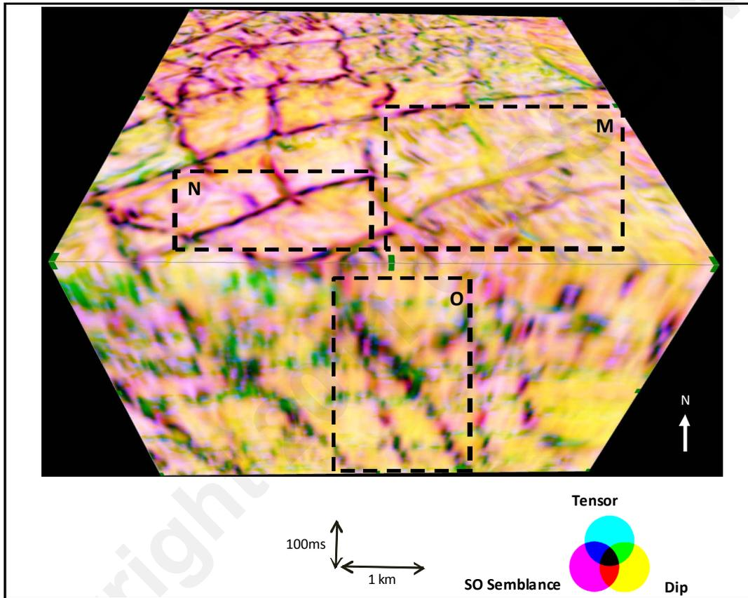
Figure 8. Volume CMY blend of structurally oriented semblance, tensor, and dip magnitude.
