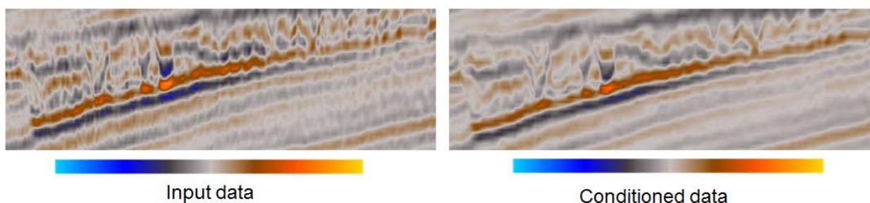
**Figure 2.** Noise Cancellation and Spectral Enhancement techniques were applied to the data, improving the imaging of the carbonate intervals while preserving the edges and subtle details of the geological features.
