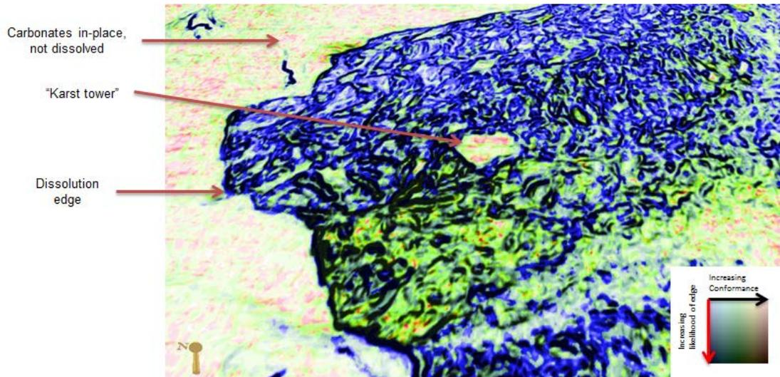
**Figure 4.** The TensorConformance combined volume highlights both the edges of the dissolution features and the nature of the infill. Carbonate pinnacles or karst towers show high Conformance values bounded by high Tensor values.
