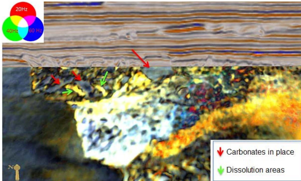
**Figure 3.** Frequency Decomposition technique based in a Matching Pursuit algorithm was applied to the dataset, and three output magnitude volumes blended on an RGB blend to highlight the dissolution features and the carbonates still in place.
