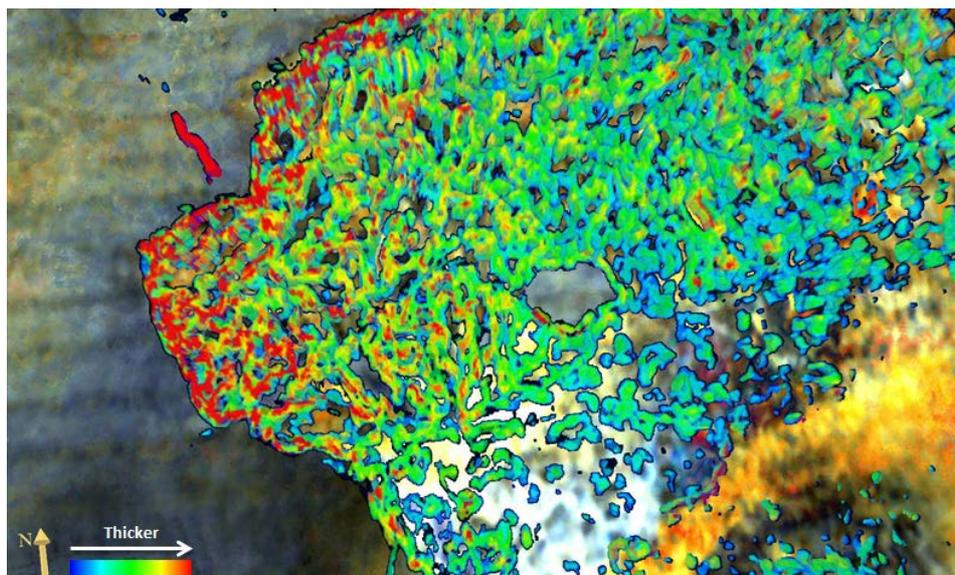
**Figure 5.** Dissolved carbonate areas were extracted using a volumetric 3D geobody colour-coded by thickness. The geobody shows a thicker dissolution on the western side, which correlates with the increase in thickness of the carbonate package towards the west.
