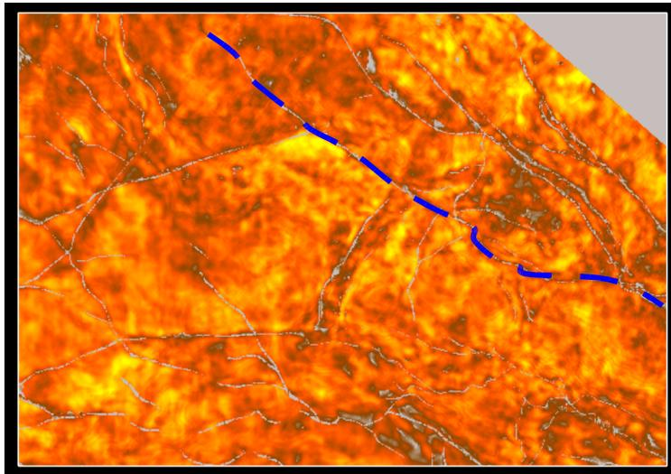
Figure 2 - A reflectivity map of the region of interest showing major interpreted fault structures. The fault section highlighted in blue is shown in isolation in a number of figures.
