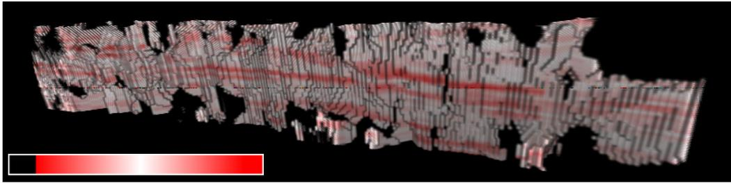
Figure 6 – A FSC indicator is computed from the difference of juxtaposed attribute statistics from the trailing and leading sides of the FDZ. Here, white bands indicate a small or no difference between the RAI values either side of the fault. Red values indicate a large difference between RAI values. Alternatively, a multi-channel rendering technique such as RGB blending (Henderson, 2007), enables the juxtaposition of RAI data from either side and from within the FDZ to be visually interpreted.
