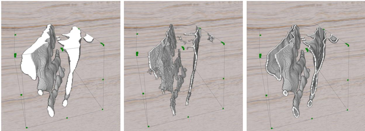
Figure 4 – The FDZ geobody region growing process results in a 3D representation of areas in the seismic reflectivity affected by faulting (*top*) as captured in the fault attribute volume.
