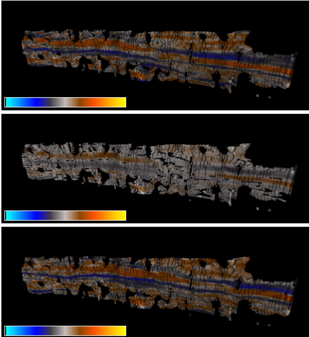
Figure 5 – As a result of the juxtaposition analysis, the local statistics of a user selected attribute are computed over the region within and the regions either side of the FDZ geobody. These statistical values are then projected across the FDZ, juxtaposing relevant values based solely on the geometry of the FDZ.
