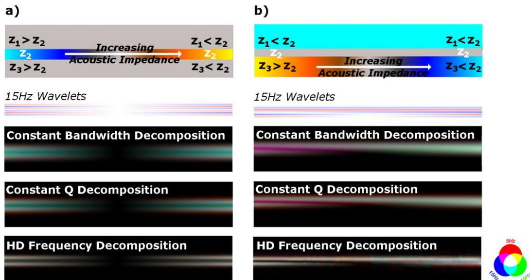
Figure 2: Impedance models, synthetic wave forms and RGB responses using different decomposition methods for a) constant thickness model with varying impedance central layer and b) constant thickness model with varying impedance lower layer.
