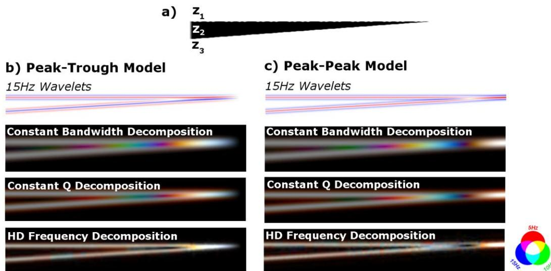
Figure 1: a) Three layer wedge model where acoustic impedance of the upper, mid and lower layers is denoted  $z_1$ ,  $z_2$  and  $z_3$  respectively; for a peak-trough model  $z_1 < z_2$  and  $z_2 > z_3$ , and for a peak-peak model  $z_1 < z_2$  and  $z_2 < z_3$ . b) and c) show synthetic models using 15Hz Ricker wavelets and their resulting RGB blends using the three magnitude volumes.
