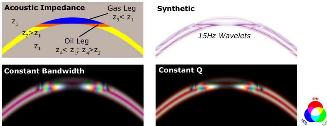
Figure 3: Impedance models, synthetic wave forms and RGB responses using different decomposition methods for structural closure models containing a) gas-water contact and b) gas-oil and oil-water contact.
